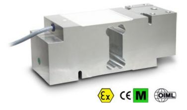
Load cells for off center loads, suitable for example to build CE-M approved scales with a single load cell; maximum platform dimensions of 800x800 mm.
