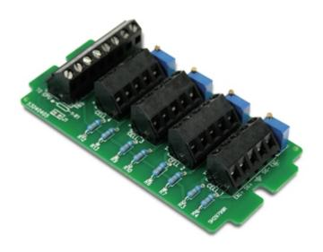
Junction and equalisation cards for up to 10 load cells. Simple to install and connect thanks to the screw terminal boards and the signal adjustment trimmers.
