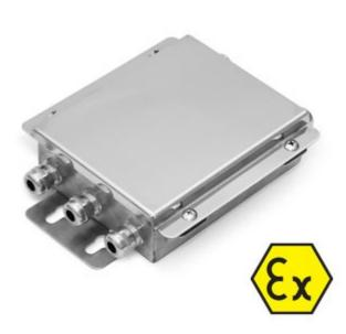
Stainless steel junction box with IP66 protection from water and dust, and fitted with an intrinsically safe electronic board for junction and equalisation of load cells. Terminal boards with screws for easing th connection of the load cells and signal adjustment trimmer, for an accurate and reliable equalisation. Marking: ATEX II 2G Ex ib IIC T6 Gb for gases. ATEX II 2D Ex tb IIIC T115°C Db IP65 for dust.
