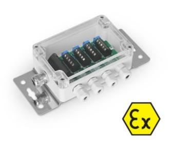
IP67 junction box fitted with electronic board for junction and equalisation of 2, 3, or 4 load cells. Terminal boards with a screw for easing the connection of the load cells and the signal adjustment trimmer, for an accurate and reliable equalisation. Marking:
