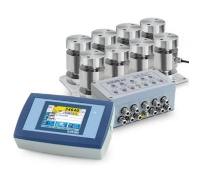
Weighbridges kit made up of 3590ET touch screen weight indicator with AF03 software for weighbridges, 6 or 8 stainless steel IP68 "RCA" analogue load cells, complete with galvanized steel oscillating resting joints and junction box with surge arresters.
