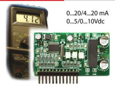
Optoisolated 16 bit analogue input, in voltage or in current. Programmable as 0...5/0...10Vdc, 0...20/4...20mA through the indicator or through the PC with Dinitools. It may be integrated in the indicators for checking the flow and dosage, for remote programming of the setpoint of hourly flow.
