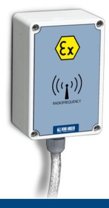
Radio frequency module for the wireless data communication in ATEX 2 and 22 zones, with protection methods according to: ATEX II 3G Ex nA IIC T6 Gc X for gases ATEX II 3D Ex tc IIIC T85°C Dc IP66 X for dust. It can be applied to both bench/floor scales as weel as mobile scales, such as pallet truck scales or pallet weighing scales, and it allows to transmit data at a very long distance.
