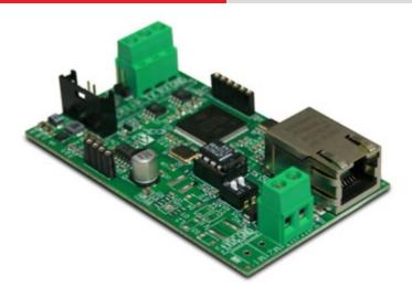
Small size, excellent signal quality, support of the most common network protocols are just a few features of this product, which allows for a network connection of any scale or weighing system to the company's computer system through the RJ45 connector; it' easy to install and it's fitted with a cable for the connection to the indicators
