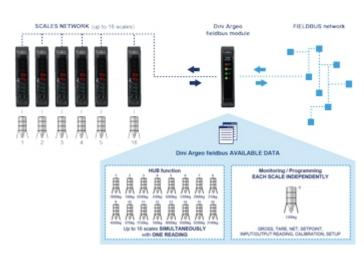
PROFINET FOR DIGITAL WEIGHING SCALES: CONFIGURATIONS (Please click on the image to enlarge)
