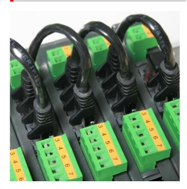
The connection between DGT1S weight transmitter and WIFIT1S module is easy and quick thanks the RS485 RJ45 connectors.
