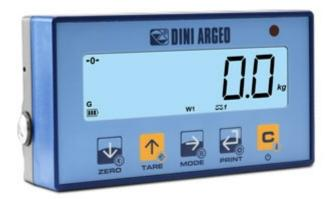
Radio frequency remote control and weight repeater in one solution, for DFW indicators and MCW crane scales. Easy to transport and view due to its small size and large backlit display. DFWPM can control the main scale functions from a distance using the integrated keypad. The USB version allows to save weights for the further processing by a PC. Fitted with a long life rechargeable battery. IP65 protection.
