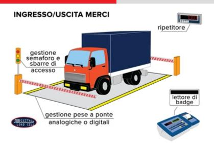
Particularly suitable for vehicle weighing and weighbridge management, with input/output control of goods. The AF03 version allows to weigh the vehicle by itself or with the trailer, either with the operator as well as self-service with the badge reader, as well as the advanced management of the data and the printouts. The AF03 also offers the possibility of managing the main digital load cells available on the market. CE-M approvable (OIML R-76 / EN 45501).
