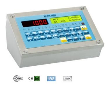
High performance digital weight indicator, with 3 serial ports, transmission protocols for data communication, completely configurable printouts, integrated alibi memory and port for connection to barcode/badge reader. The wide range of connectable accessories and printers guarantees the maximum interfaceability and versatility. CE-M approvable (OIML R-76 / EN 45501).
